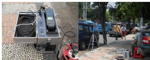
Figure 9. Measurement of Ambient Air Pollutant (CO) Using Ecoline 6000 Gas Analyzer
