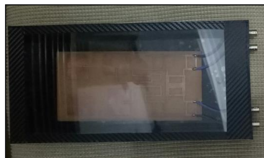
Figure 21 Final Prototype of Smart Antenna
