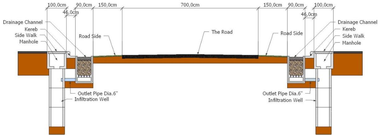
Figure 5: Typical Cross Section of the Road
