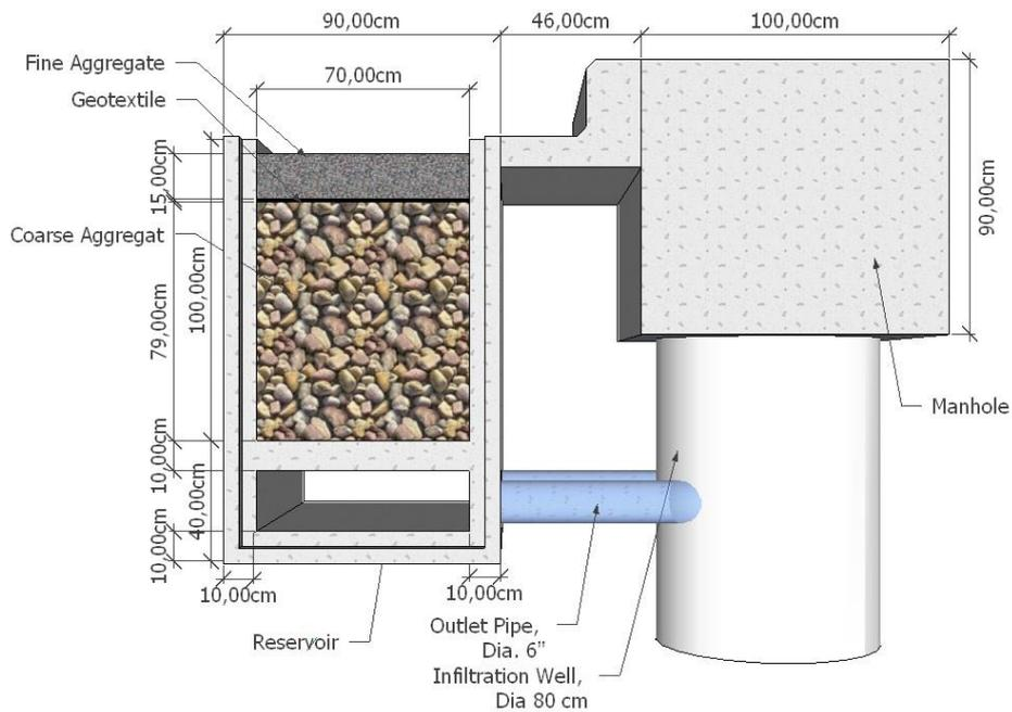
Figure 6: Typical Details of Channels and Infiltration Wells
