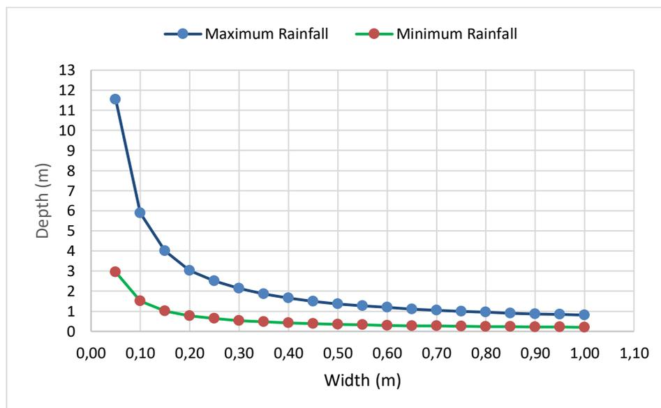
Figure 4: Graph of the Relationship of Width and Aggregate Depth for Maximum and Minimum Rainfall.
